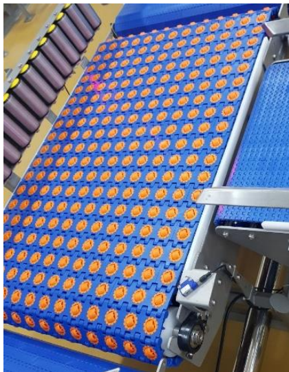
Plastic & Roller Conveyor
